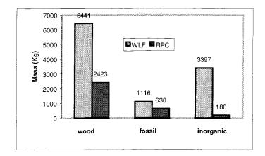
Fig. 6. Resource consumption per category for WLF and RPC systems (using more material derived from wood for the WLF system)
