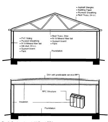
Fig. 3. Sections through WLF and RPC systems
