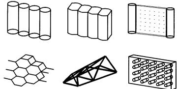
Fig. 2. RPC: Potential structural systems
